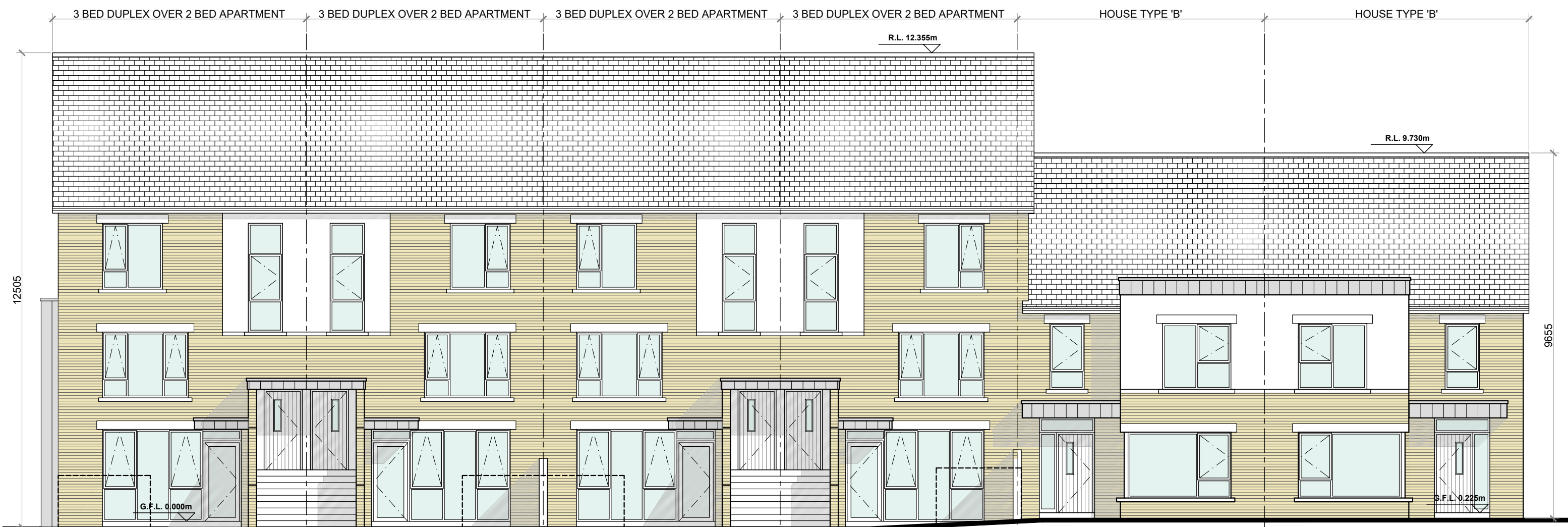
FRONT ELEVATION @ 1:100 DUPLEX BLOCK TYPE 4A
