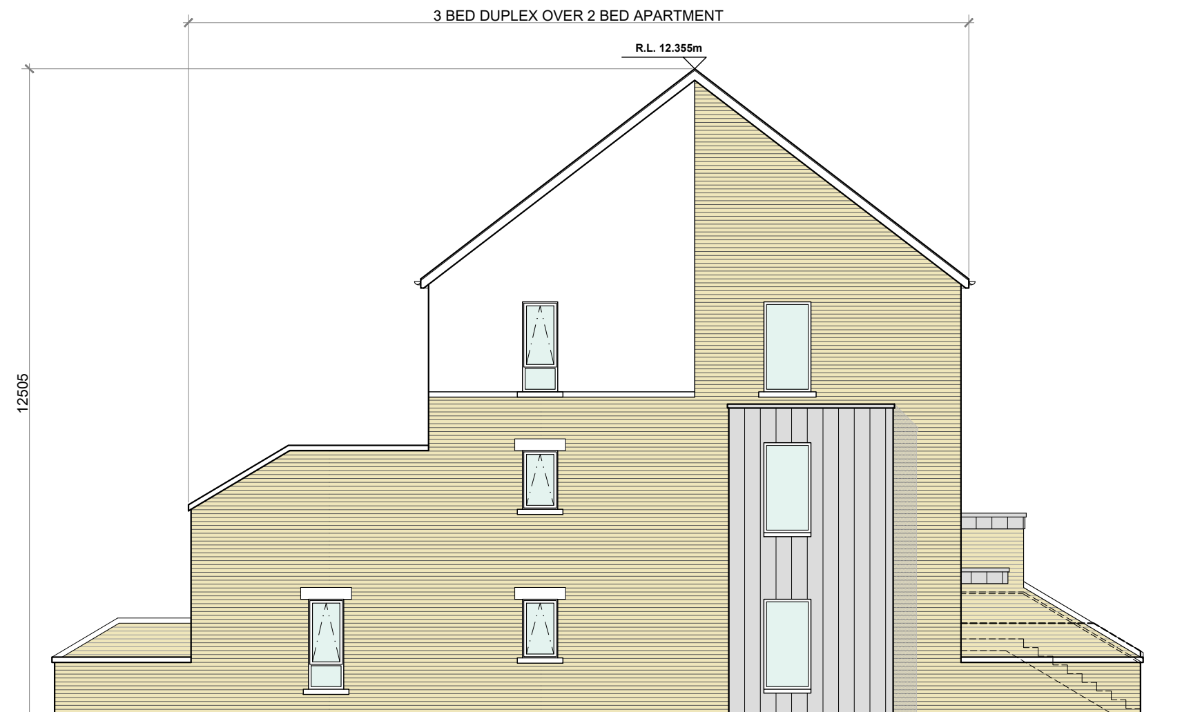
SIDE (DUAL FRONTAGE) ELEVATION @ 1:100 DUPLEX BLOCK TYPE 4A
