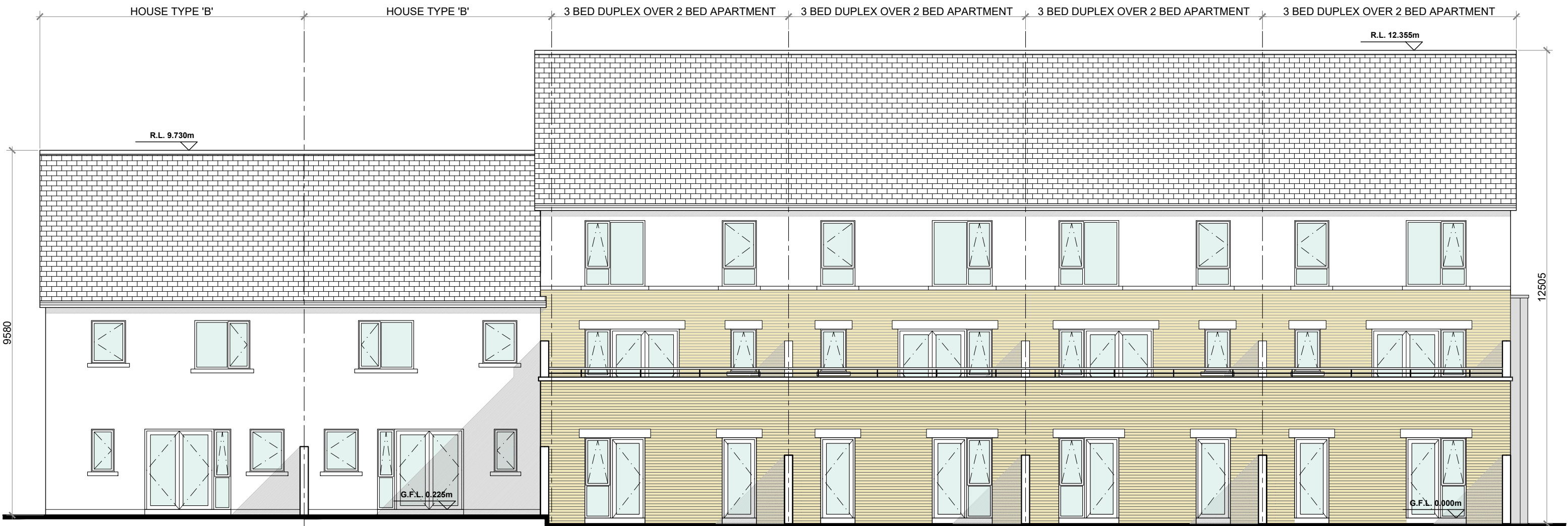
REAR ELEVATION @ 1:100 DUPLEX BLOCK TYPE 4A
